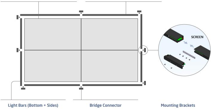
Each bar contains an array of IR LEDs to provide a light source for object detection.
